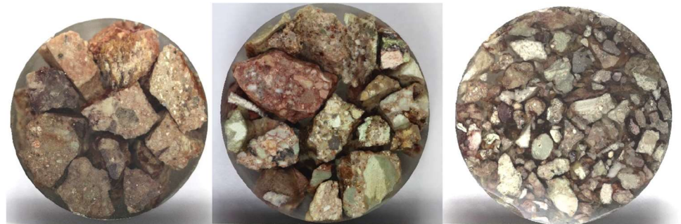
Figure 1: Examples of 40-mm Polished Block sections; from left to right: +9000 fraction, +4500 fraction, +1000 fraction. Scale is in millimeters. Note the details of particles becoming available through this method.
